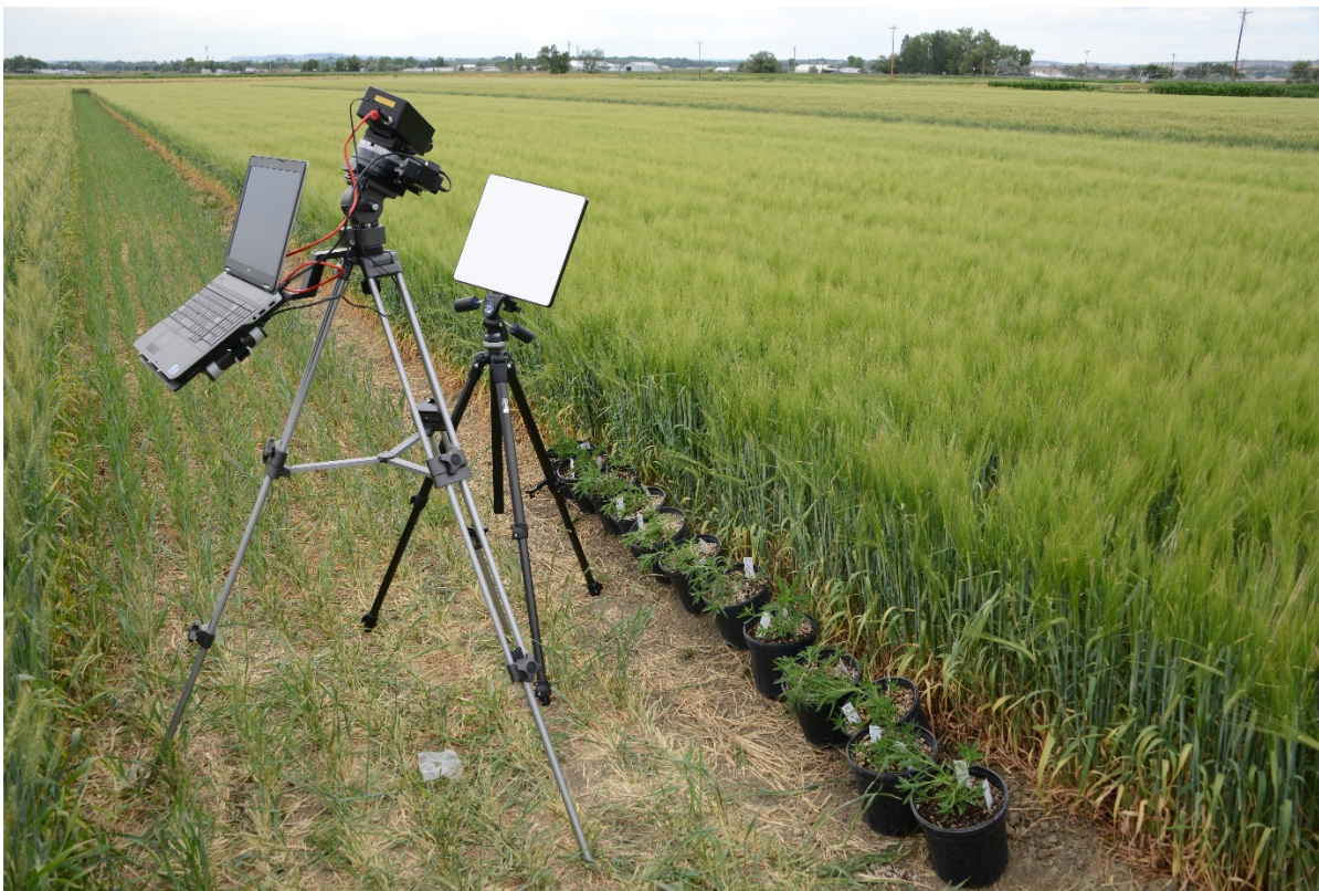
Figure 1: Tripod-mounted hyperspectral imager recording pixel-to-pixel variations by viewing a high-reflectance calibration plate prior to recording spectral images of the potted weeds and crops.
