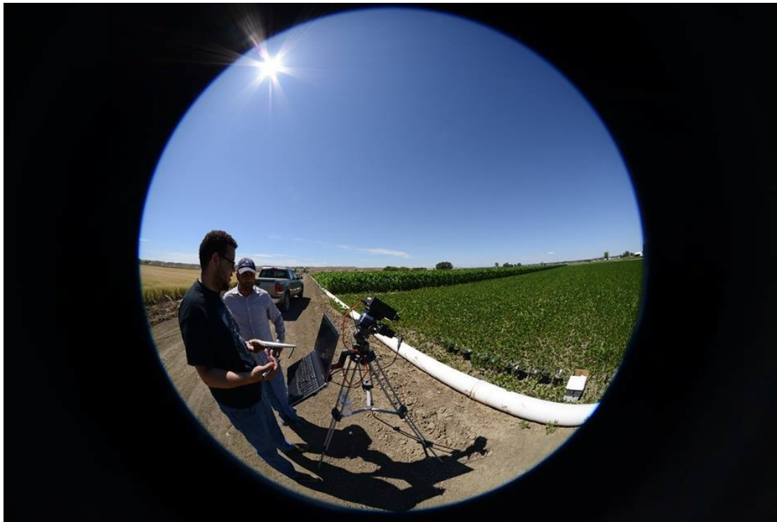
Figure 4. Fisheye photograph of the hyperspectral imager scanning across the potted weeds in a field of soybeans under a clear sky with direct sunlight.
