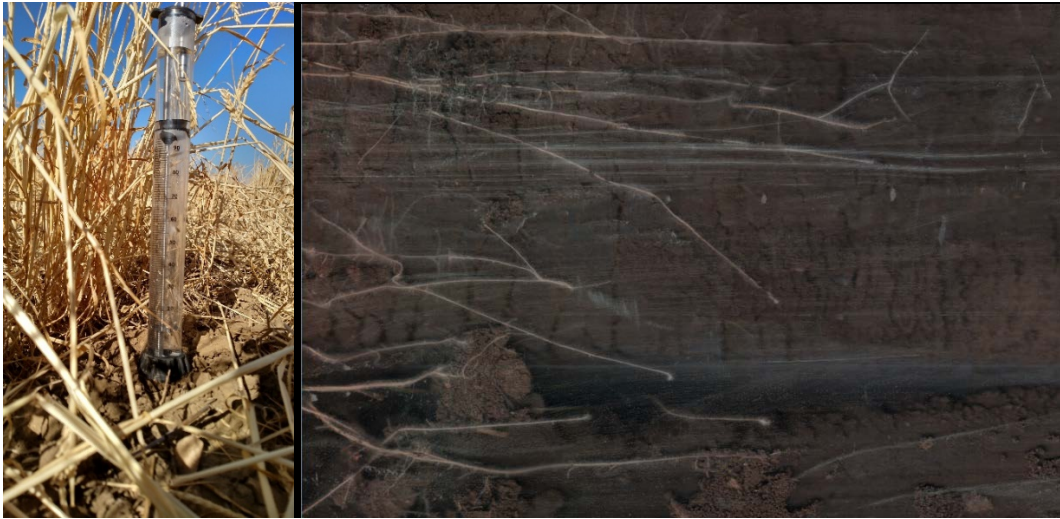
Figure 2. Infiltrometer measurements investigating how fast the soil can take water after cover crop termination. Right hand picture is of a root scan collected with a minirhizotron (below ground camera) to monitor underground root profile differences just prior to termination of the cover crops.
